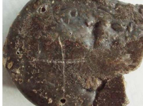
Fig 7. Composite from mixture „ Ash+ PET”(volume of ash 22% )
