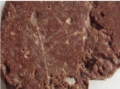
Fig. 5. Composite from mixture „Clay +PET”. 50% (mass), a-white clay , b- brown clay
