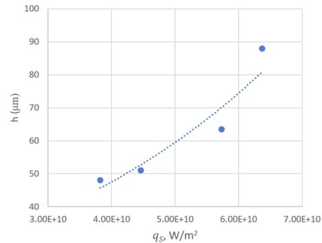
Fig. 10. Graph shows depth changes as a function from power density  $h=h(q_s)$ . All other parameters are constant:  $f=2$  [kHz],  $v=5$  [mm/s],  $\tau=200$  [ns].
