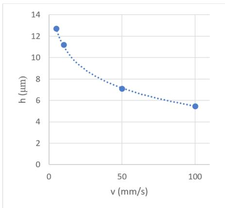
Fig. 8. Graph shows depth changes as a function from marking speed  $h=h(v)$ . Variable parameter is  $\tau$ . All other parameters are constant:  $f=2$  [kHz],  $k_p=80$  [%],  $\tau=200$  [ns].
