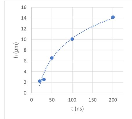
Fig. 6. Graph shows depth changes as a function from impulse length  $h=h(\tau)$ . Variable parameter is  $\tau$ . All other parameters are constant:  $f = 2$  [kHz],  $k_p = 80$  [%],  $v = 20$  [mm/s].  $k_p$  – mean power [%];  $\tau$  – pulse duration [ns];  $f$  – pulse frequency [kHz];  $v$  – marking speed [mm/s]
