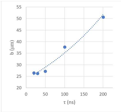
Fig. 7. Graph shows width changes as a function from impulse length  $b=b(\tau)$ . Variable parameter is  $\tau$ . All other parameters are constant:  $f=2$  [kHz],  $k_p=80$  [%],  $v=20$  [mm/s].
