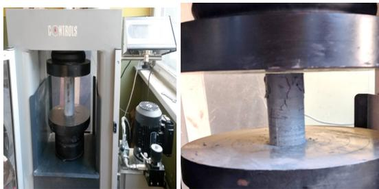
Fig. 1. Specimen compressive strength test.
