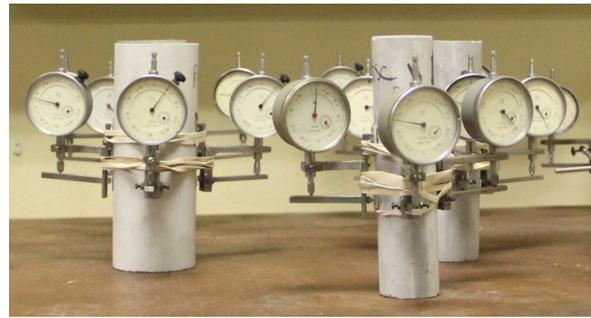
Fig. 3. Specimens prepared for shrinkage testing.
