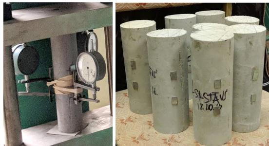
Fig. 2. Specimens prepared for creep testing.
