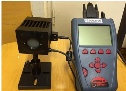
Fig. 8. Power measurement sensor OPHIR F150A-BB-26
