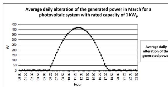
Fig. 4. Average daily power output change in March for a photovoltaic system with a rated power of 1.0 kW<sub>p</sub>, obtained by PVGIS-CMSAF
