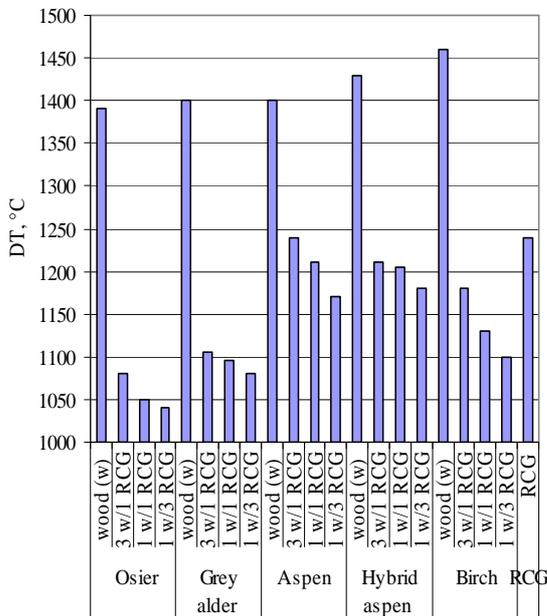
Fig. 1. Deformation temperature (DT) of various energy crops and their mixtures: w- the particular species of wood, RCG – reed canary grass
