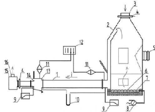
Fig. 1. Pilot unit: 1- settling element; 2- airing cupboard; 3- pipe union under ASO – 3 measurement; 4 - chimney valve flow control regulator with screw; 5 – pressurized hung sleeve; 6 – atometer; 7 - heater; 8 - current controller; 9 – mictomanometer; 10 - U-type magnahelic gauge; 11 – allonge; 12 – portable rotary device; 13 – storage of equal static pressure; 14 – collector; 15 – blower unit; 16 –air extraction pipe to the atmosphere.
