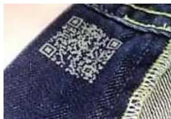
Fig. 13. 2D matrix code directly on the article [44].
