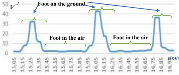
Fig. 2. A signal fragment produced by one sensor.
