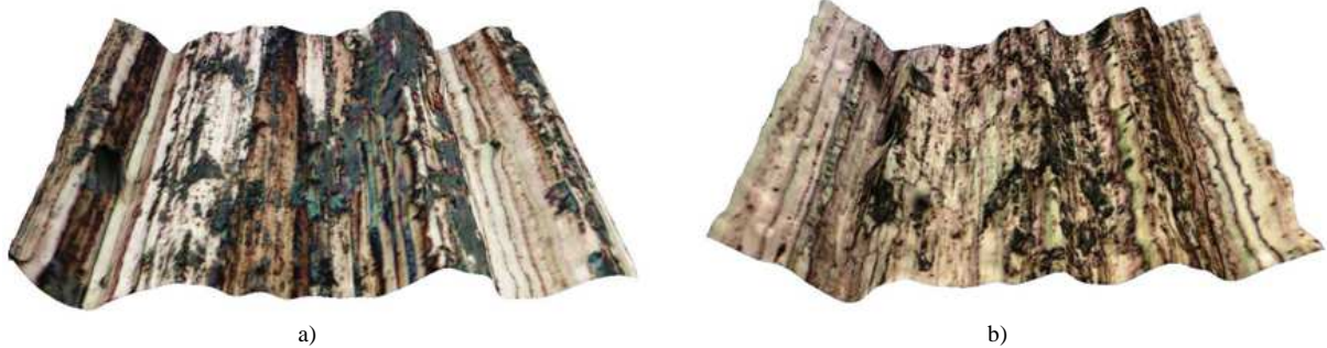
Fig. 5 The 3-D microphotography of the machined surfaces: a – the traditional technology ( v = \text{const} ); b – the proposed grinding technology with variable cutting speed ( v = \text{var} )
