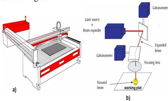
Fig.5. a) plotter system b) scanner system
