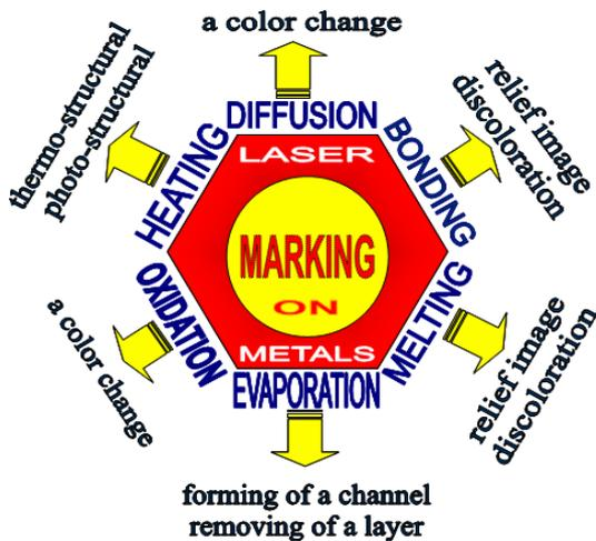
Fig. 2. Physical processes in laser marking on metals
