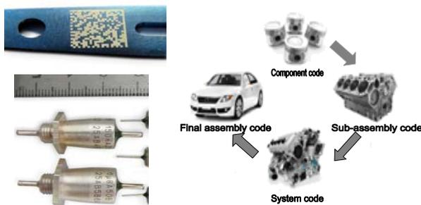
Fig. 1. Laser marking of parts with different codes
