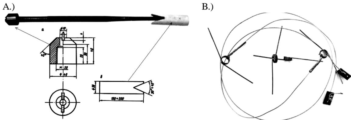
Fig. 3. Bench-mark station (A.; Fig.2,nr.5) for installation in floor and rope-bench-mark stations (B.) for installation in roof (B.; Fig.2,nr.4)
