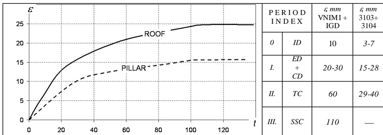
Fig. 5. Roof-to-floor convergence curves and comparison table for deformation by VNIMI+IGD and received experimental data
