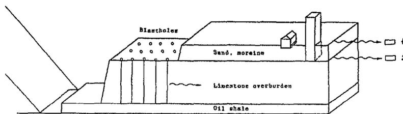
Figure 1. Ground vibration measurements of overburden blast in oil shale surface mining:
