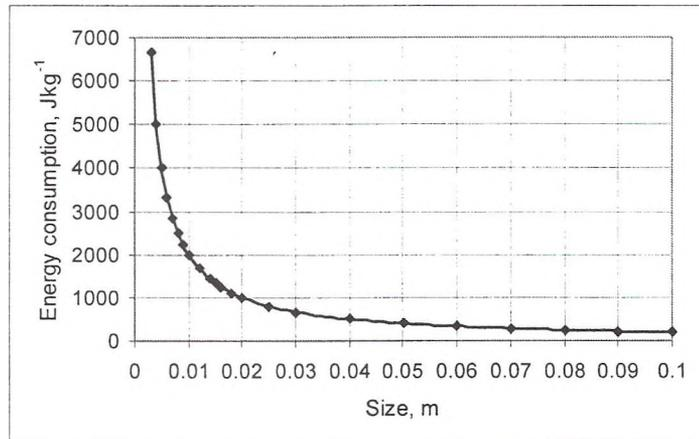
Fig.4. Energy consumption for common reed cutting
