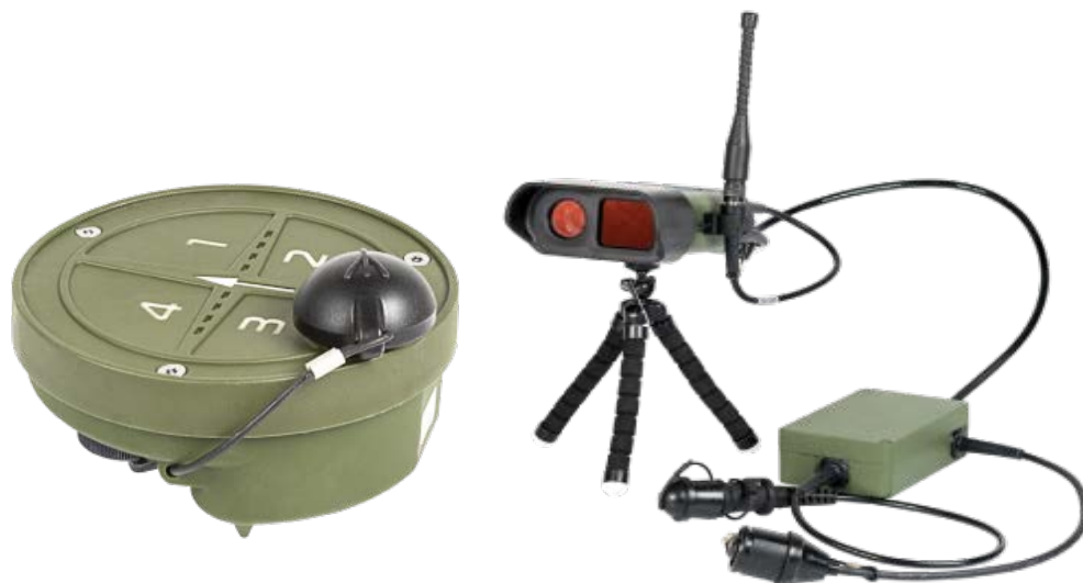
Fig.4 Components of the DEFENGUARD presence detection system (compiled by the authors)
