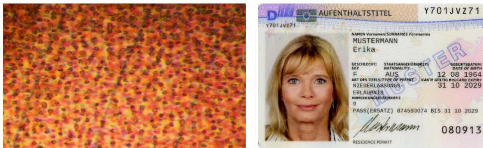
Fig.8 Polymer-adapted inkjet printing on polymer documents (Source: DPR, 2022)
