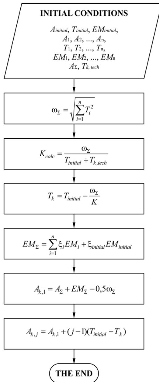
Figure 2 Algorithm for dimensioning units with non-adjustable compensators
