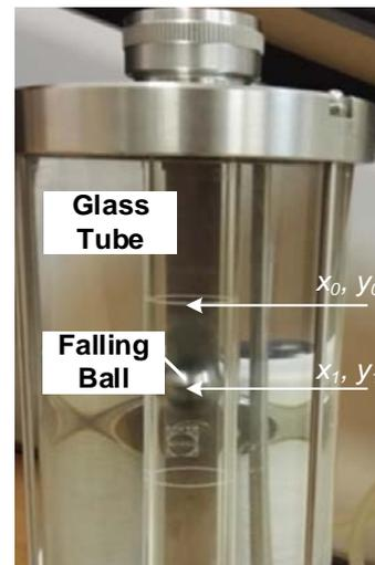
Figure 3 The structure of the viscometer with liquid
