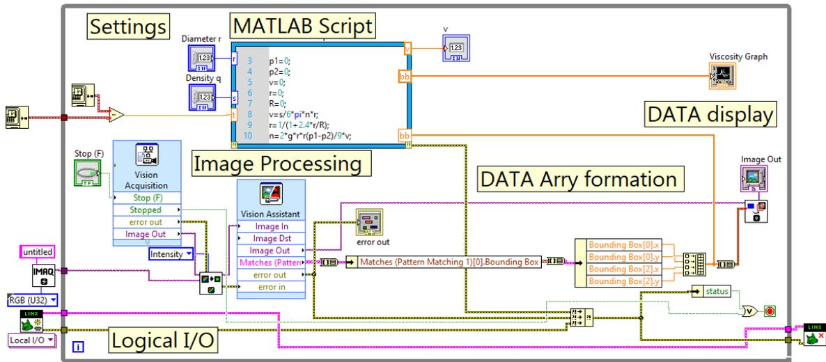
Figure 8 The LabVIEW diagram of the measurement system
