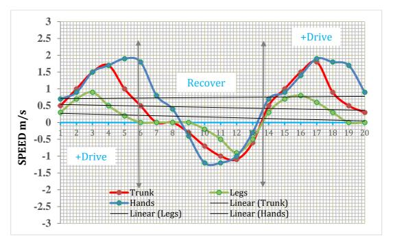
Figure 3 Movement speed of the trunk, legs and hands in one stroke cycle
