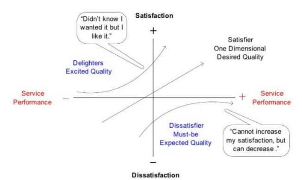
Fig. 2 Kano's model: three main categories of factors (attributes) affecting customers' perception of the offered service *(Source: Kano, 1996)*
