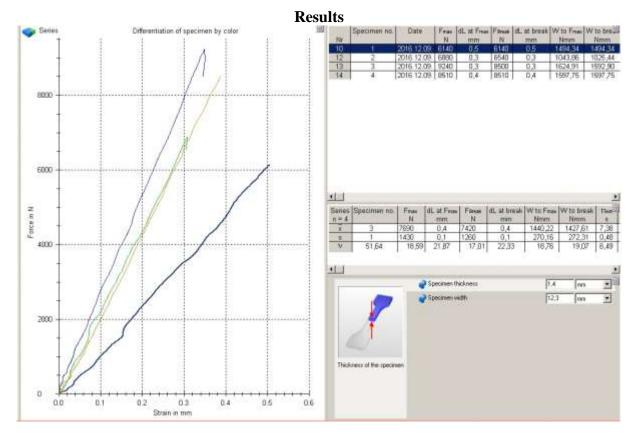
Fig. 1 Showed tensile strengh for carbon fiber with mechanical cut and laser cut
