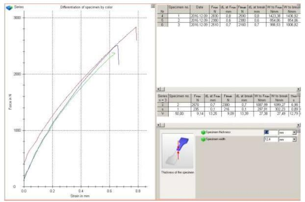
Fig.3 Showed tensile strengh for glass and flax fiber
