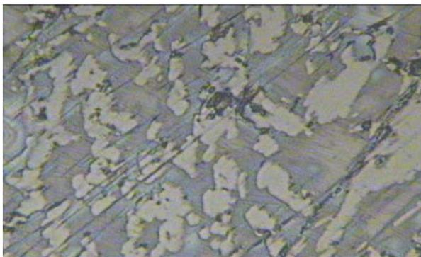
Fig. 8. I layer - Chromium carbides + metal base – x500
