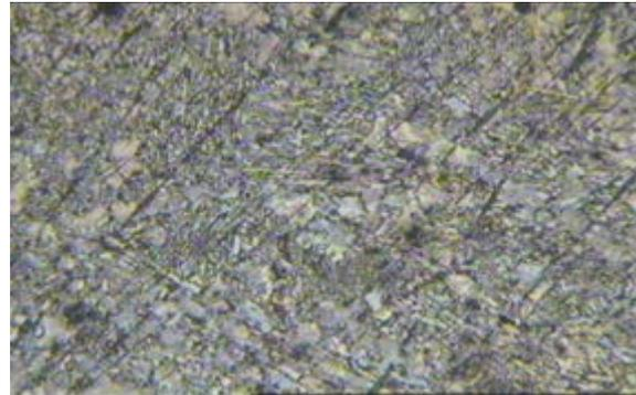
Fig. 5. I layer - Chromium carbides + metal base - x50
