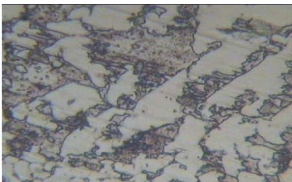
Fig. 9. I layer - Chromium carbides + metal base – x1000
