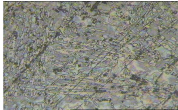
Fig. 6. I layer - Chromium carbides + metal base – x100
