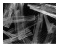
Fig.4. Fibers of polypropylene "FiberMesh 300"
