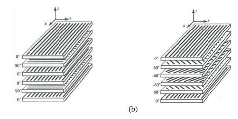
*Fig.2.* Arrangement of plies in (a) a crossply laminate and (b) an angle-ply laminate sandwiched between 0° plies [8]
