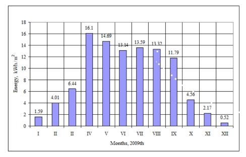
Fig.9. The recorded output (the batteries are not loaded) energy levels in 2009th, Total 101.9  $\rm kWh/m^2$
