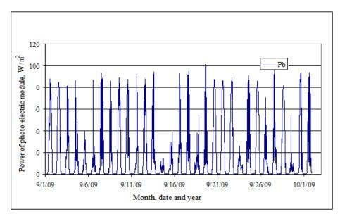
*Fig.7.* Photo-electric power module diagram and power diagram energy output in September, 2009<sup>th</sup>
