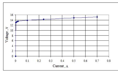
Fig.3. Photo-electric module, power recorders Volt-Ampere characteristic
