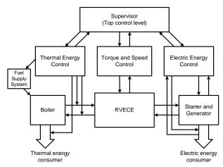
Fig. 2. Cogeneration plant control system.
