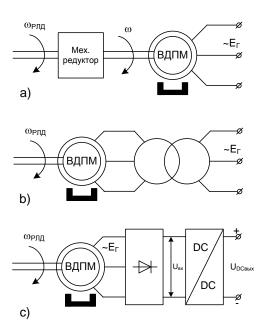
Fig. 5. Different options of speed or output generator voltage multipliers.
