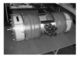
Fig. 1. Rotary-vane external combustion engine.
