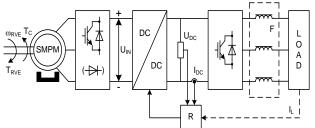
Fig. 9. The structure of the electric part with PFC-module.
