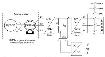
Fig. 4. The structure of the electrical subsystem of the autonomous power supply system based on rotary-vane external combustion engine.
