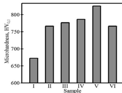
Fig.4. Dependence of the microhardness HV<sub>0,1</sub> of the metal matrix on the boron content in high chromium white cast iron
