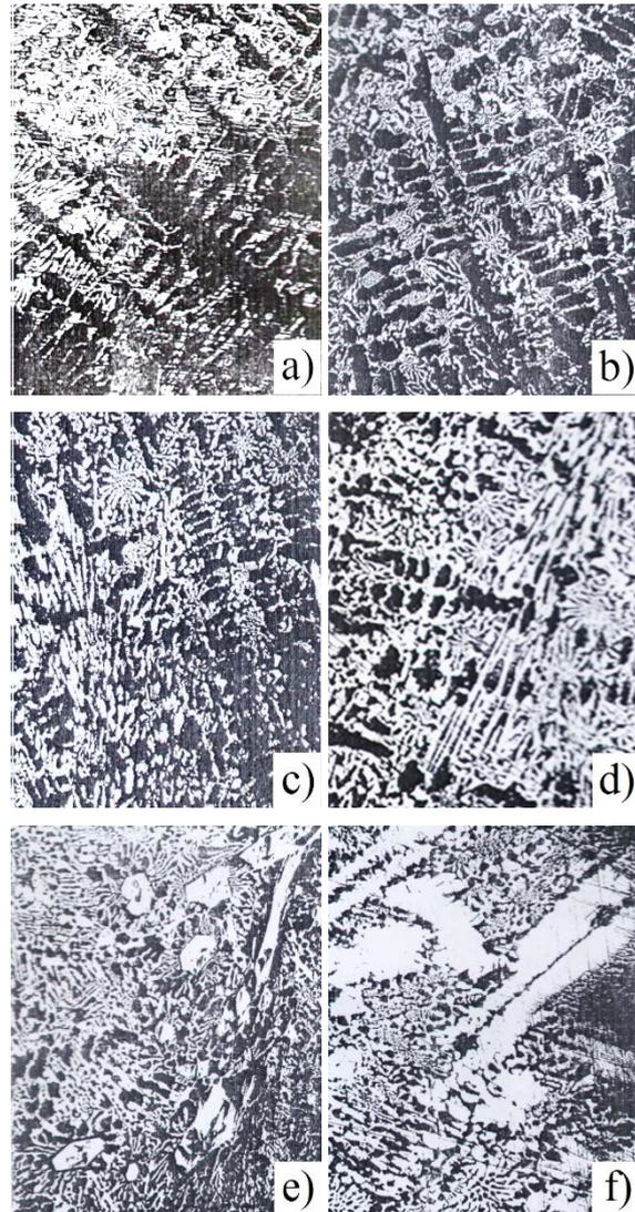
Fig.1. Microstructure of high chromium white cast irons alloyed with boron x100. a) - 0% B; b) - 0,18% B; c) - 0,23% B; d) - 0,59% B; e) - 0,96% B; f) - 1,25% B
