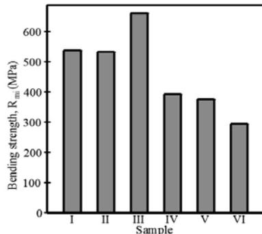
Fig.3. Dependence of the bending strength R<sub>mi</sub> on the boron content in high chromium white cast iron
