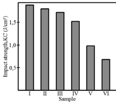
Fig.2. Dependence of the impact toughness KC on the boron content in high chromium white cast iron
