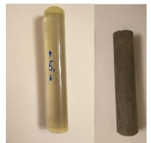
Fig 1. Experimental samples of polyurethane material before and after dynamic processing
