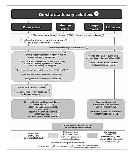
Fig. 2. On-site stationary instruments and methods for determining water discharge classification with (the best quality image can be viewed on the website of the State Hydrological Institute (SHI) [7])
