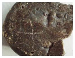
Fig 7. Composite from mixture " Ash+ PET"(volume of ash 22% )
