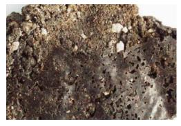
Fig. 4. Composite from mixture "Clay + PET". PET content 30% (mass)
