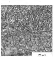
Fig.4. Microstructure of the austempered ductile iron sample with coating Ni+TiN after heat treatment at 290°C, 6 h
