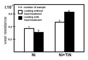
Fig.5. Wear resistance I of the coatings composition Ni (samples 1 and 2) and composition Ni+TiN (samples 3 and 4), deposited on the austempered ductile iron samples.
