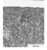
Fig.3. Microstructure of the austempered ductile iron sample with coatings Ni after heat treatment at 290°C, 6 h
