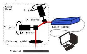
Fig. 4. Schematic view of Rofin powerline f20 experimental set-up
