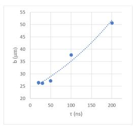
Fig. 7. Graph shows width changes as a function from impulse length  $b=b(\tau)$ . Variable parameter is  $\tau$ . All other parameters are constant:  $f=2 \text{ [kHz]}, k_p = 80 \text{ [\%]}, v=20 \text{ [mm/s]}.$
