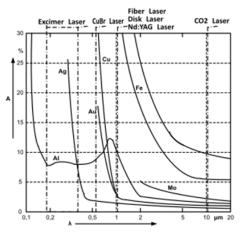
Fig. 3. Various material electromagnetic radiation absobrtion [%] depending on emited wavelength [ $\mu$ m].
