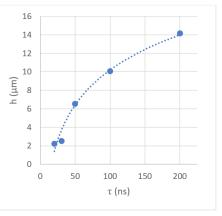
Fig. 6. Graph shows depth changes as a function from impulse length h=h(τ). Variable parameter is τ. All other parameters are constant: f= 2 [kHz], k<sub>p</sub> = 80 [%], v=20 [mm/s]. k<sub>p</sub> – mean power [%]; τ – pulse duration [ns]; f – pulse frequency [kHz]; v – marking speed [mm/s]
