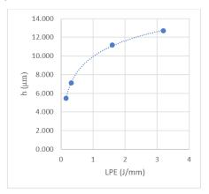
Fig. 11. Graph shows depth changes as a function from linear pulse energy. All other parameters are constant: f= 2 [kHz], v = 5 [mm/s], τ=200 [ns], P=18 [W].
