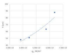
Fig. 10. Graph shows depth changes as a function from power density  $h=h(q_s)$ . All other parameters are constant: f=2 [kHz], v = 5 [mm/s],  $\tau=200$  [ns].
