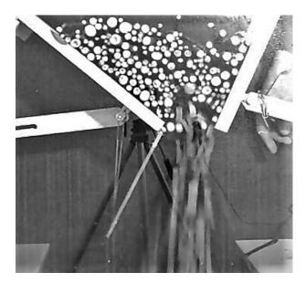
Fig. 4. .The normal character of energy willow cuttings flow inSAE-UP research
