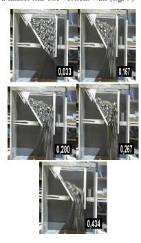
Fig. 2. Theflowphaseof energy willow cuttings from the hoppers if theslanted corners of half-planesare $\alpha$ =90° и  $\beta$ =40°
