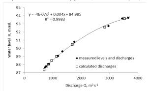
Fig. 2. The stage-discharge relationship curve for the Daugava River at Daugavpils for the spring floods of 2007-2017 (main data source: LVGMC).
