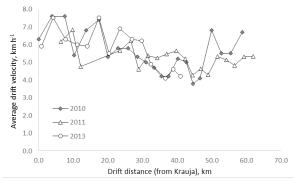
Fig. 5. Variation of the average drift velocity in the Daugava River downstream from Krauja during the spring floods of 2010, 2011 and 2013.
