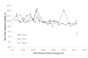
Fig. 6. Variation of the main channel's depth in the Daugava River downstream from Krauja during the spring floods of 2010, 2011 and 2013.
