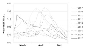
Fig. 1. Fluctuation of water levels in the Daugava River at Daugavpils during the spring floods of 2007-2017 (dates of the drift experiments are marked as empty curves; data source: LVGMC).
