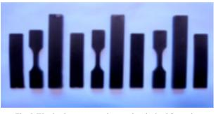
Fig. 5. Wood polymer composite samples obtained for testing
