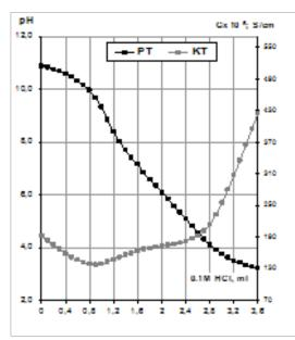
Fig. 2. Curves of potentiometric and conductometric titration of a 0.01% PEI water solution
