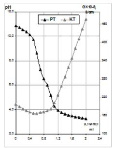
Fig. 1. Curves of potentiometric and conductometric titration of a 0.01% HASL water solution
