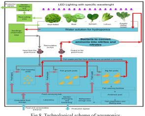
Fig.8. Technological scheme of aquaponics (LEDGROW Engineering Ltd.)
