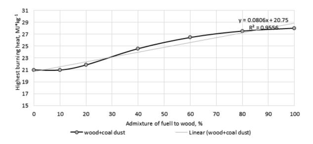
Fig.7. Highest burning heat of composit biomas fuel, wood+coal dust.
