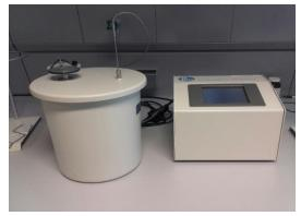
Fig.4. Oxygen bomb calorimeter Paar 6772. The highest heat of combustion was determined using dry samples. Three parallel measurements were made for each sample and measurement errors were calculated.
