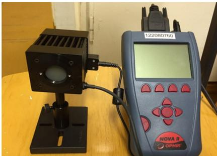
Fig. 8. Power measurement sensor OPHIR F150A-BB-26
