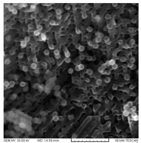
SEM HV: 30.00 kV WD: 14.59 mm Line VEGAN TESCAN View field: 7.204 µm Det SE Detector 2 µm Daugavpils University Fig. 2. SEM image of the defect region of the Ag / opal composite.
