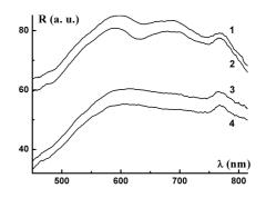
Fig. 3. Reflectance spectra of silica opal template (1, 2) and those of nanocomposite Ag / opal (3, 4) at the angles of incidence  $25^{o}$  (1, 3) and  $30^{o}$  (2, 4).
