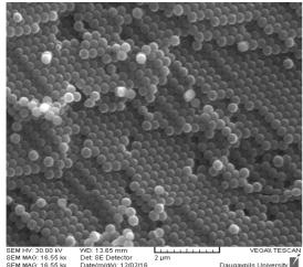
SEM MAG: 18.55 kx Date(m/dy): 12/02/16 Daugavpills Universit Fig. 1. SEM image of the silica opal matrix under study.
