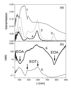
Fig. 5. (a) Transmission spectra of the monolayer ( $T_1(\lambda)$ , curve 1), plasmonic-photonic crystal Ag / ML / Ag ( $T_2(\lambda)$  curve 2), microresonator ( $T_3(\lambda)$ , curve 3), plasmonic-photonic crystal with microresonator Ag / cavity / Ag / ML / Ag, ( $T_4(\lambda)$ , curve 4) at the normal light incidence  $\theta = 0^\circ$ . (b) The ratios  $r_5(\lambda) = T_2(\lambda)/T_1(\lambda)$  (curve 5),  $r_5(\lambda) = T_4(\lambda)/(T_2(\lambda) \times T_3(\lambda))$  (curve 6).
