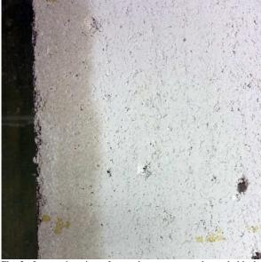
Fig. 3. Intersection view of aerated concrete wetted sample block after dosage of 441 ml sprayed water during 23 min– the penetration of water into the deeper surface areas is visible up to  $\sim$ 4 cm.
