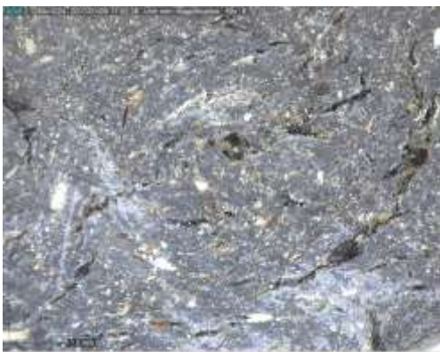
Fig.11. Sapropel structure (polished surface) after heat treatment at t=20°C
