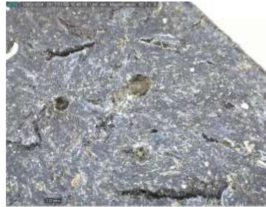
Fig.12. Sapropel structure after 20 min heat treatment at t=150°C
