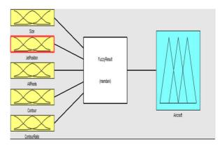
Fig. 2. Block diagram of the system for decision making by means of the Mamdani method, built in Matlab.
