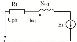
Fig.4. Electrical equivalent circuit for one motor phase
