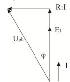
Fig.3. Phasor diagram for the maximum thrust
