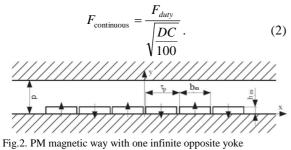
Output parameter for the calculation of the linear motor magnetic system shown in Fig. 2 is the value of magnetic flux density in the air gap. In order to derive an analytical equation for its calculation, the PM magnetic way must be modeled. This is done by replacing each PM with two current densities of different signs. After using the image theory both  $B_x$ and  $B_{\rm v}$  components of the magnetic flux density are obtained.
