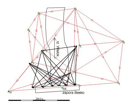
Fig. 1. A conventional geodetic control network
