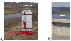
*Fig. 2.* Construction of points in a geodetic control network (during GPS survey): a - a reference point, b - a point on a copping of the water damming object
