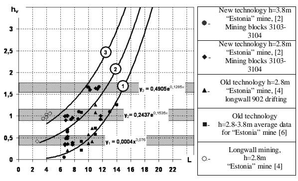
*Fig.* 7. The exfoliation depth  $(h_v)$  dependence on the critical area (L) *Where, geological conditions classification by the roof stability:* ①*-stable;* ②*- average;* ③*- weak.*
