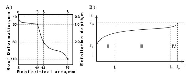
*Fig. 4.* Roof-to-floor convergence curve by the VNIMI and IGD data (A.) and typical curve for long-term stability analysis (B.) [3]
