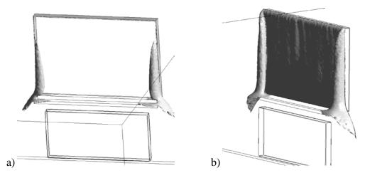
*Fig.* 8. Isosurfaces of v=0,55 m/s (a) and  $T=7^{\circ}$ C (b) for modelling variant 3-1
