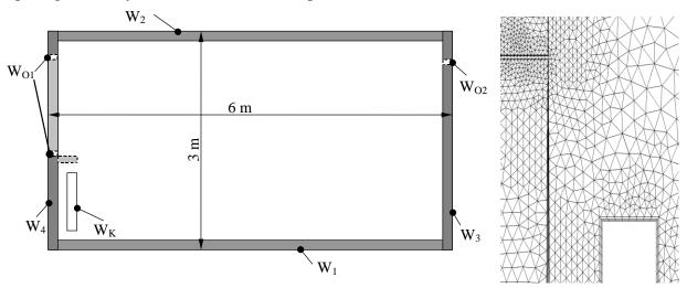
Fig. 1. Layout of building structures in a room and illustration of discretisation
