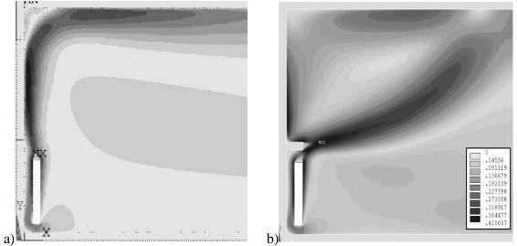
*Fig. 3.* Stationary distribution of the velocity modulus in the modelled room. Images (a) and (b) correspond to variants 1-1 and 1-2 respectively
