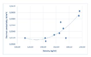
Fig.2. Thermal conductivity/density graph
