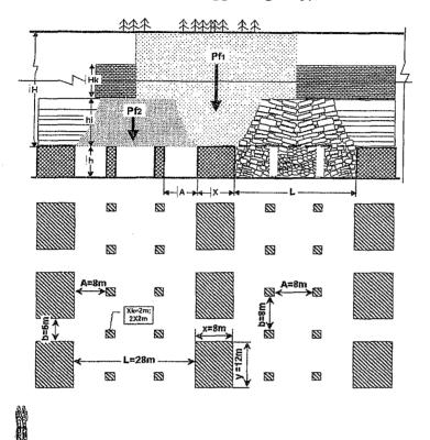
Where: x, y -the pillar dimensions, m; A, b - rooms sizes, m; H - covered rocks thickness, m; S -cross-sectional area of a pillar,m<sup>2</sup>;  $\gamma$ -the covered rocks average density (for Estonian oil shale mines  $\gamma = 0,025$ ), MPa/m; k<sub>k</sub>-factor of the pillar form; q -factor of the pillar sides destruction, when blasting works are presented, then q=0,6m, and when CM using q=0; n - the given factor of pillars safety.
