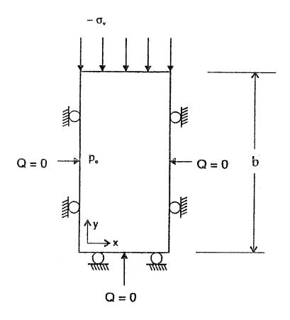
$\sigma v$  - applied vertical pressure;  $p_o$  - initial excess pore pressure; Q - outflow (inflow) rate of water; b - thickness of the stratum.
