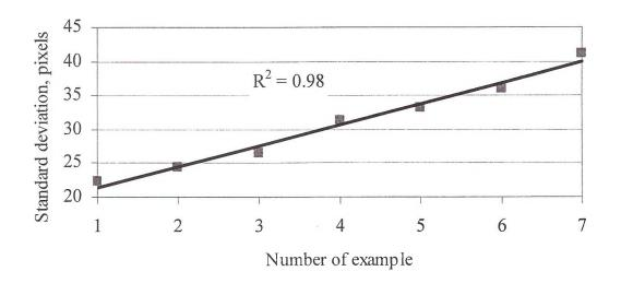
Fig.2. Standard deviation of distances between particles
