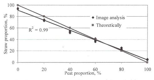
Fig.3. Comparison data of Image analyze and theoretical data
