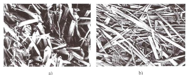
*Fig.1.* Orientation of stalks in a straw bale
