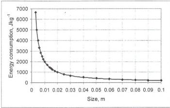
Fig.4. Energy consumption for common reed cutting
