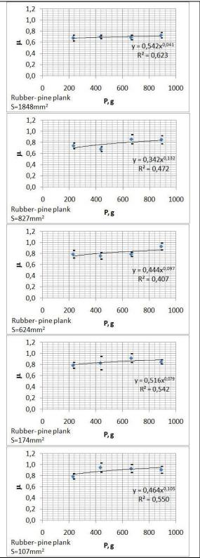
*Fig.2.* Dependence of sliding friction coefficient between rubber and pine plank on weight for different contact surface areas
